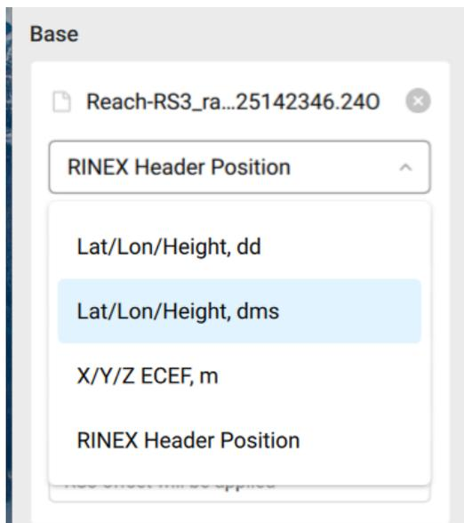
5. Enter the latitude, longitude, and ellipsoid height values from your OPUS solution here.
