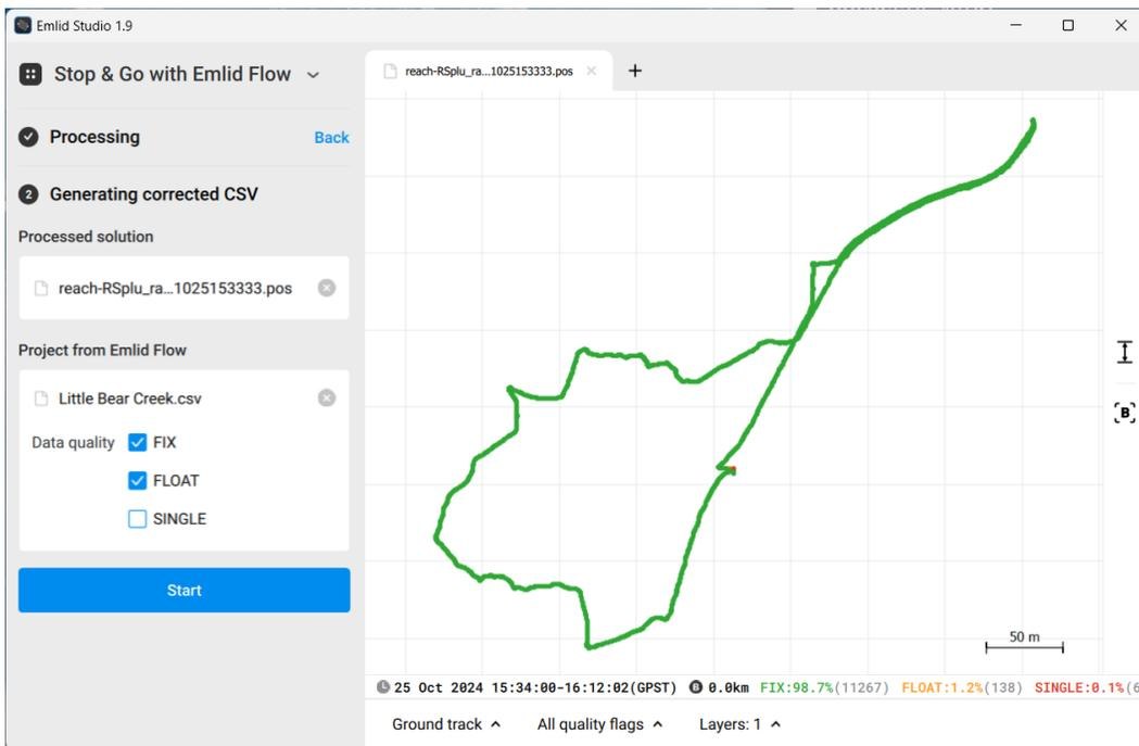
7. Next, add the GCP file exported from the Emlid Flow app. Click **Start** to post-process the GCP points from the corrected log file. The resulting map will show the corrected point locations according to their status. A CSV file of the corrected points will also be generated (by default in the same directory as the rover log file).
