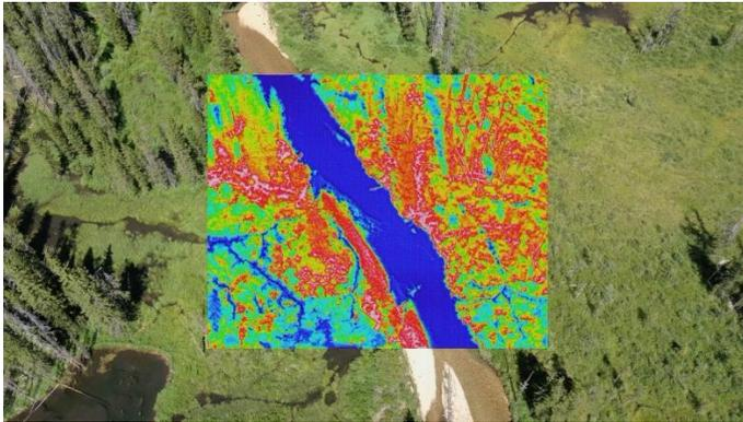
*Difference in image extent for thermal and RGB camera on the Autel Evo II Dual drone*
