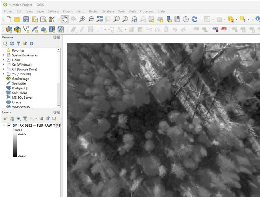
For photogrammetric processing of the images, we need: 1) R-JPEG images that record the actual TIR or temperature values, and 2) a photogrammetric application (like Metashape!) that can recognize R-JPEG formats and import the temperature/TIR layer.
