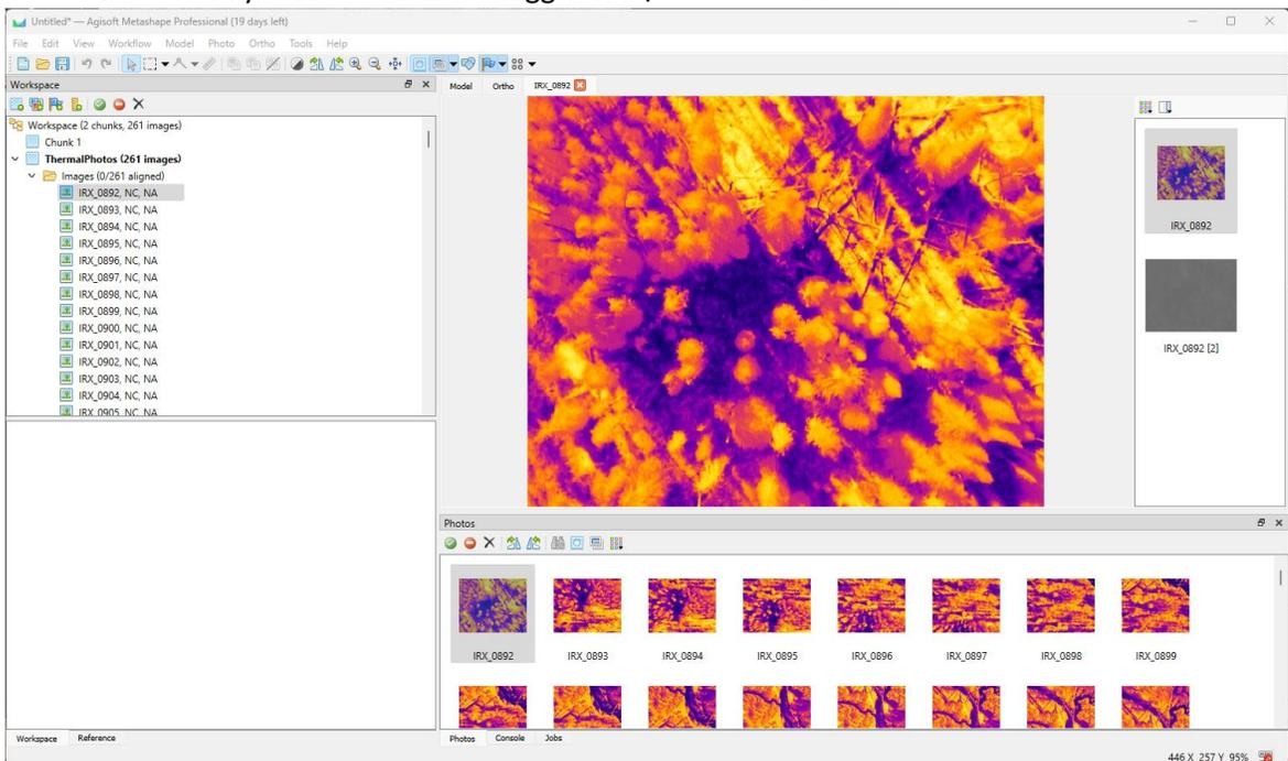
4. Photogrammetric applications like Metashape can sometimes have issues estimating camera interior orientation parameters like focal length from TIR images. This can result in difficulty aligning photos. One way to help with this is to tell Metashape what the camera focal length is.
