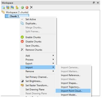
2. Make sure the projection is set correctly (UTM 11 – EPSG::32611) and that the "Use as laser scans" option is checked. Then click OK to import the lidar data. It may take a minute or two to load the data.
