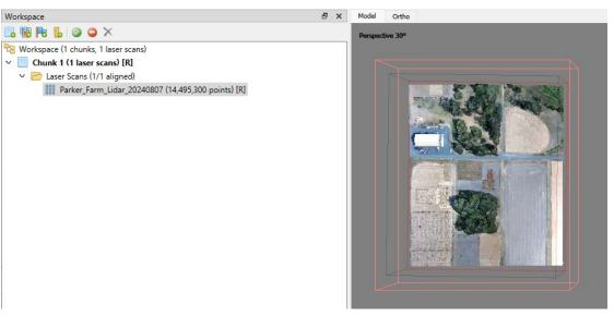
4. Change to the Reference window and import the ground control points for Parker Farm. Make sure the field names line up correctly with the data (i.e., the correct column numbers are being used for import) for the ground control file and that import starts on line 2 (to avoid importing the header row), and click OK. Click Yes to All to create markers for the ground control points.
