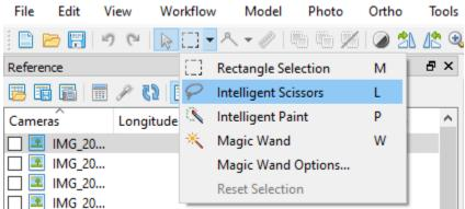
3. Use the Intelligent Scissors tool to digitize a polygon around the circle of the turntable, staying on the white part. No need to be super precise here, just get the basic shape.
